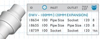
Our most recently introduced Combination Joints (18634, 18635 & 18739) allow for 40 degrees inclusive swivel movement and accommodate up to a large 120mm expansion. For installations where a full 120mm expansion is not necessary, we also offer a product range with a smaller expansion of up to 52mm. Other options for DWV and HDPE pipework are also available.
